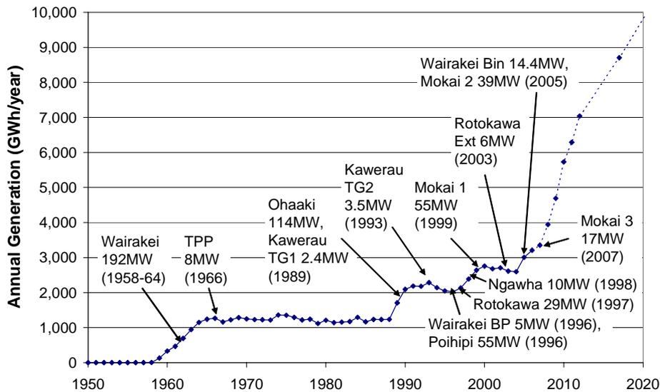
**Figure 1:** Historical and Projected Growth in Geothermal Electricity Generation in New Zealand. Source: Historical generation – MED 2007; station capacities and commissioning years – NZGA website [www.nzgeothermal.org.nz](http://www.nzgeothermal.org.nz); projections – based on advised capacities and dates for current developments and an assumption that a total 1000 MWe additional capacity will be installed by 2025.
