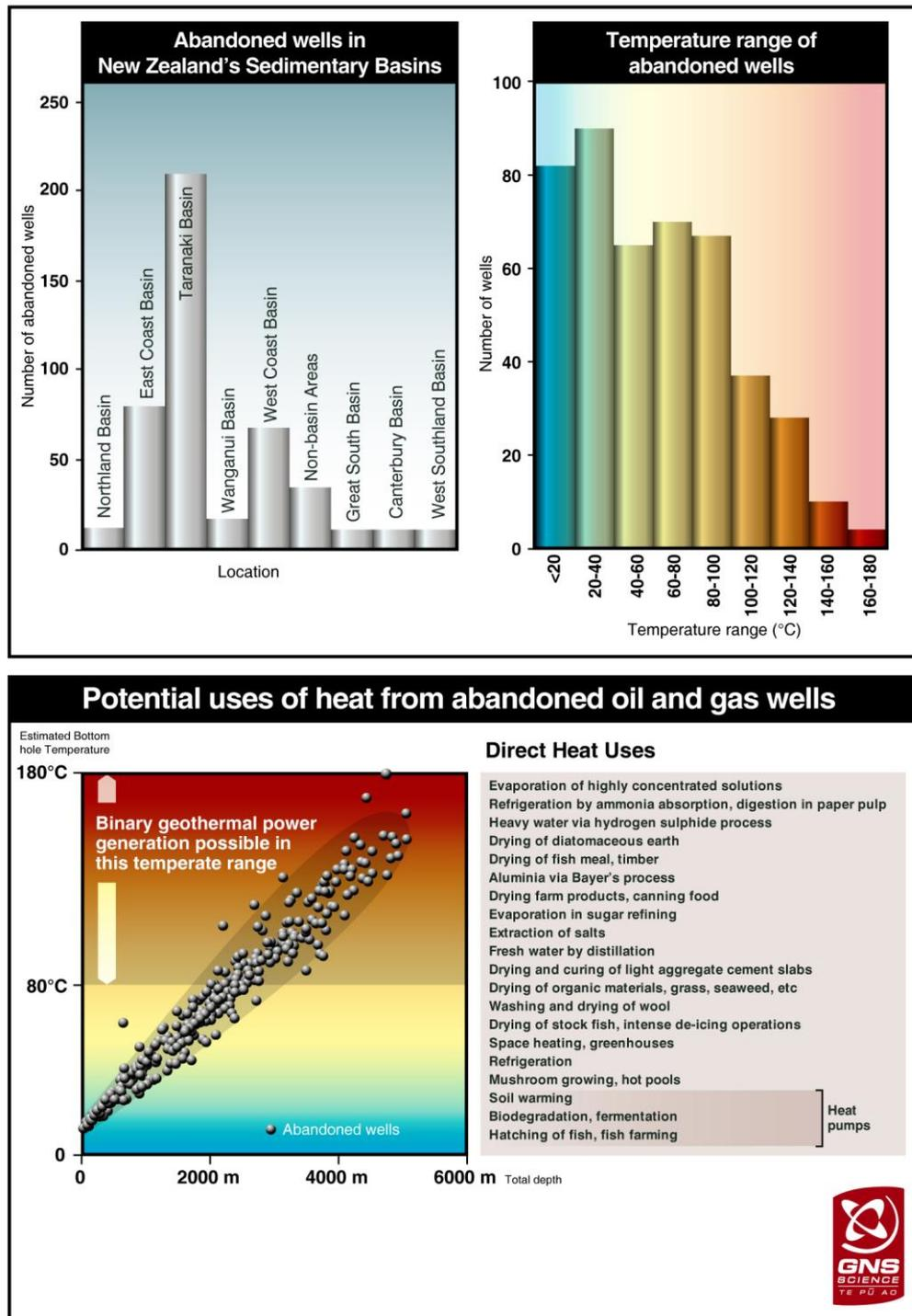
Figure 2.4. Abandoned hydrocarbon wells in offshore<sup>18</sup> and onshore New Zealand showing the number of wells in various basins, temperatures and possible geothermal uses (Reyes 2007).
