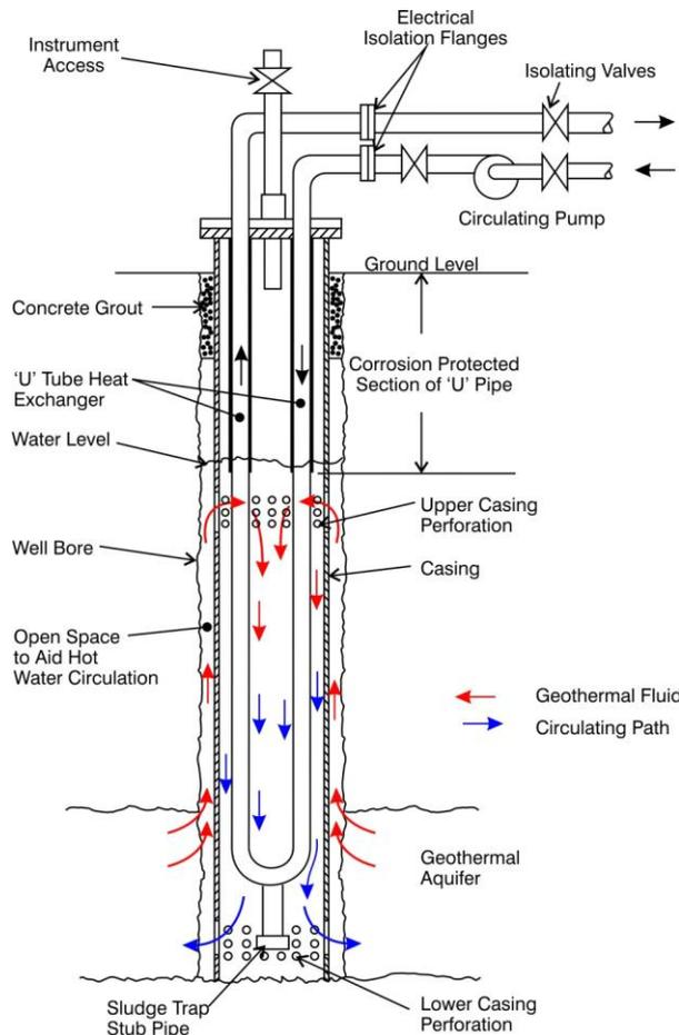
**Figure 3.3:** Typical down-hole heat exchanger with promoter tube casing (Thain et al 2006)
