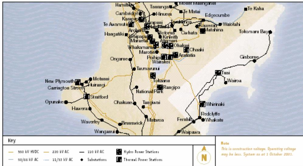
The present system has a single-circuit 110 kV line from Tuai to Fernhill and a double-circuit 110 kV line from Tuai to Redclyffe. Options to rationalise the present configuration are being investigated in preparation for life extension work that is scheduled to begin on the assets.
