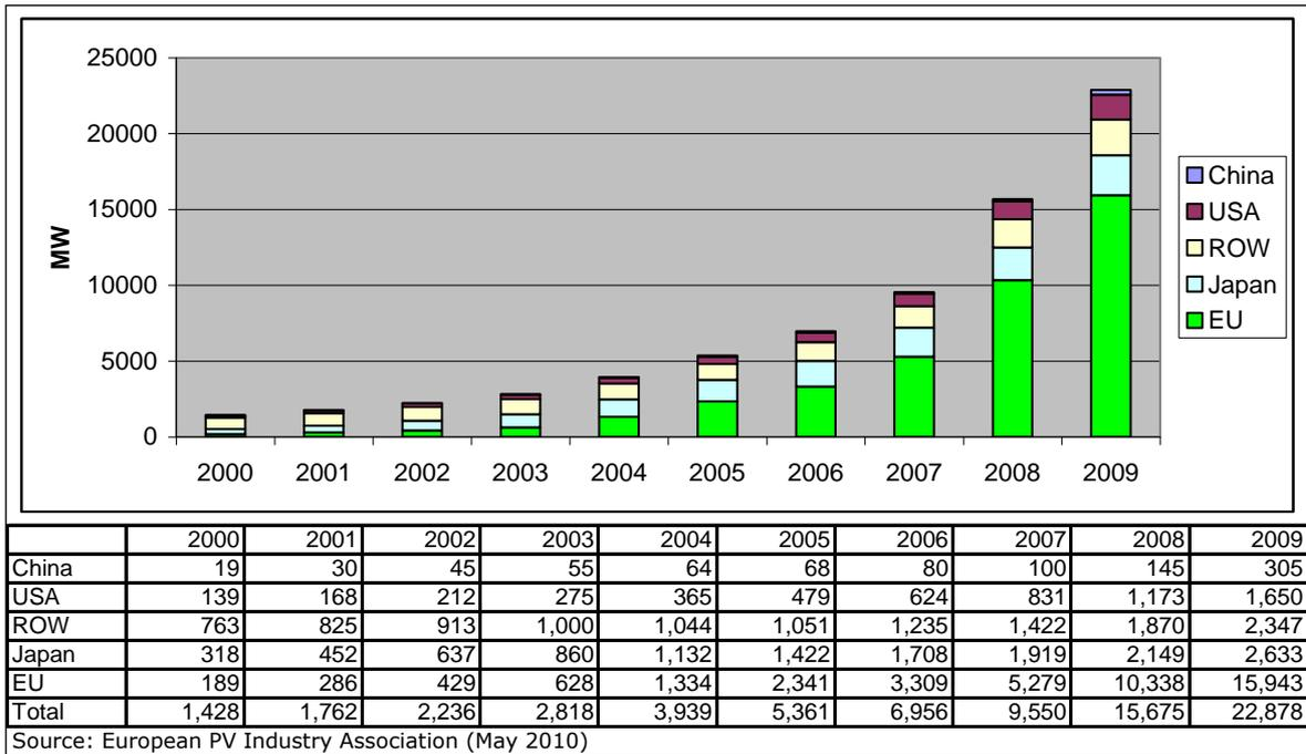
**Figure 3:** Historical development of World cumulative PV power installed in main geographies
