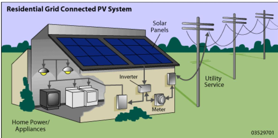
**Figure 2:** Residential Grid Connected PV system
