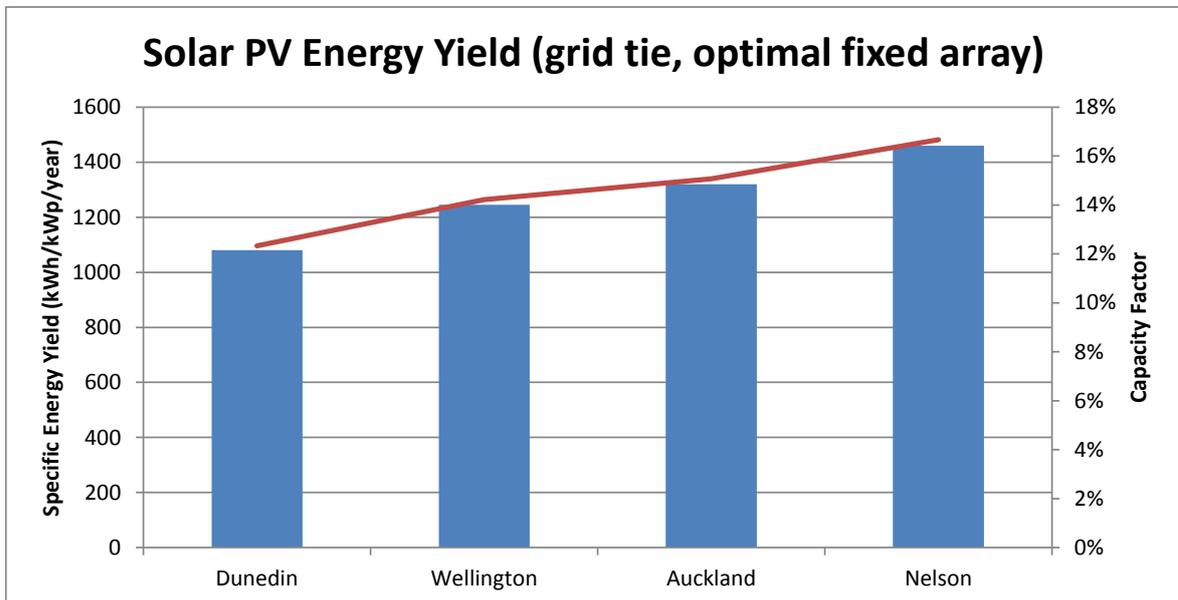
**Figure 6:** Expected annual specific energy yield for fixed grid connected PV arrays in New Zealand
