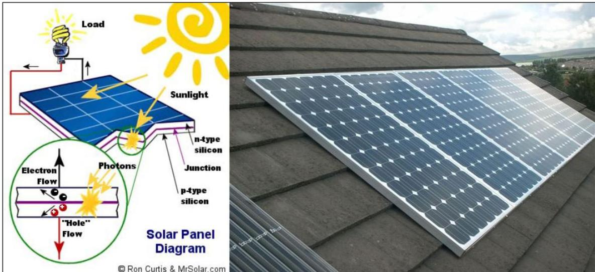
**Figure 1:** Solar panel diagram and installed on residential roof
