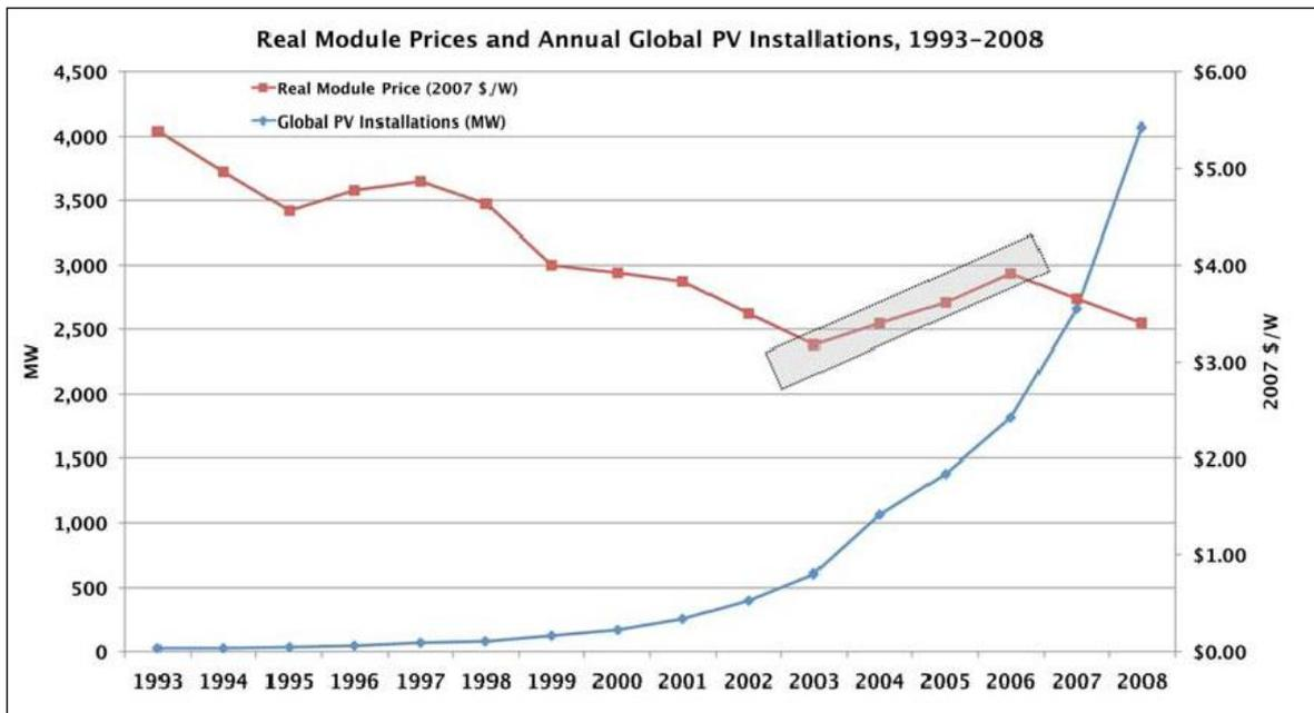
**Figure 5:** Real PV Module Prices (\$US) and Annual Global PV Installations, 1993-2008<sup>8</sup>
