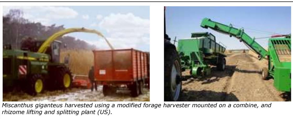
*Miscanthus giganteus harvested using a modified forage harvester mounted on a combine, and rhizome lifting and splitting plant (US).*
